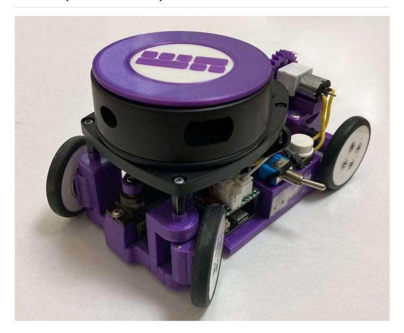
A robot designed to solve the WRO FutureEngineers 2021 task (Version Mk. IV)
